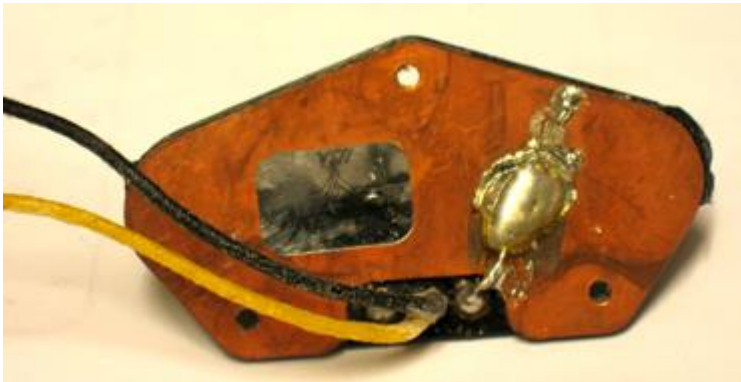
Figure 2. Telecaster bridge pickup. With this model, the black wire is connected to the base plate. For some switch positions, this connection must be disconnected and the base plate is then connected via an additional wire to the earth/ground.
