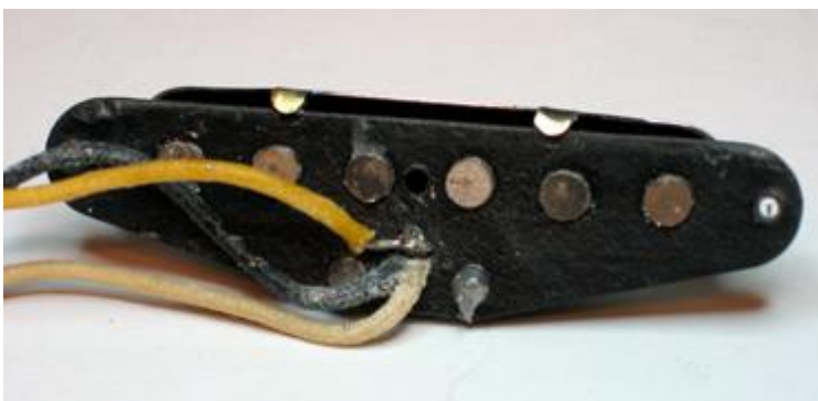
Figure 2. Telecaster bridge pickup. With this model, the black wire is connected to the base plate. For some switch positions, this connection must be disconnected and the base plate is then connected via an additional wire to the earth/ground.
